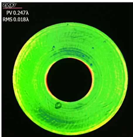
Fig. 6. RMS figure error of the PM with coating.
