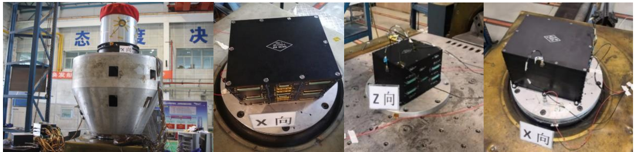
Figure 21. Vibration test photo of VT main body, Video processing box, Electric box and TEC controller box (from left to right)
